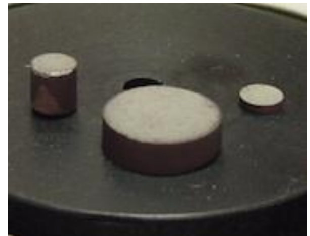
Samples of \text{U}_3\text{Si}_5 prepared via powder metallurgy route for property analysis
